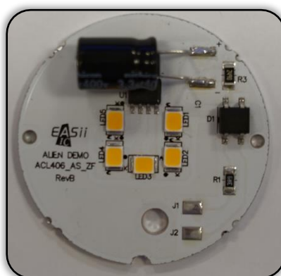
Figure 4: PCBA with Zero Flicker for the ACL406AS at 230V AC IMS PCB, diameter 40 mm, thickness 1.6mm.
