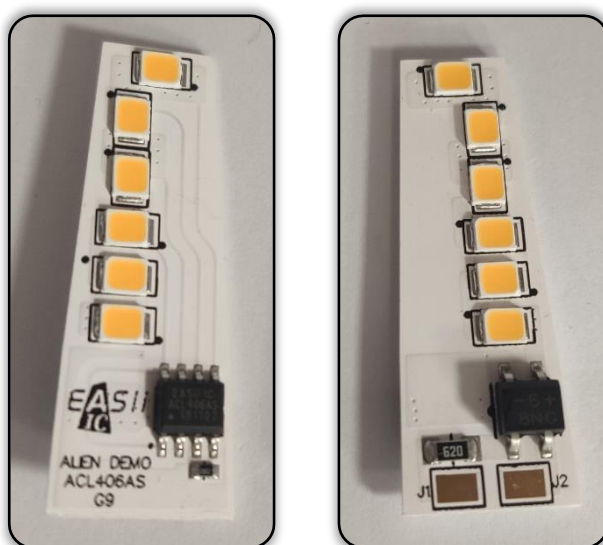
Figure 3: G9 light PCBA with ACL406AS at 230V AC CEM3 PCB, size 37 x 13 mm, thickness 1.6 mm.
